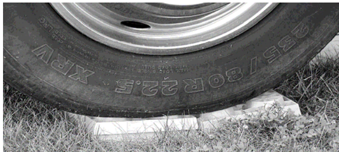
The blocks used in this photo have raised circular sections that do not evenly distribute the weight over the tire's footprint.
